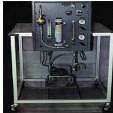
Temporary Mobile Stack monitor
