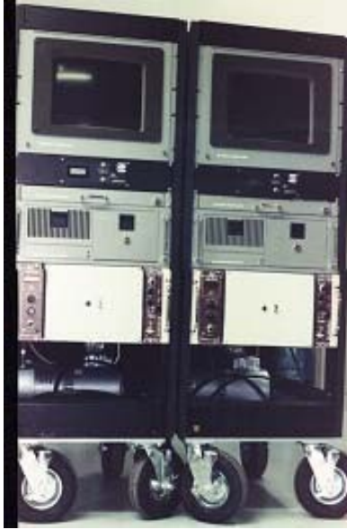
Cart-Mounted Control System for Stack Monitors
