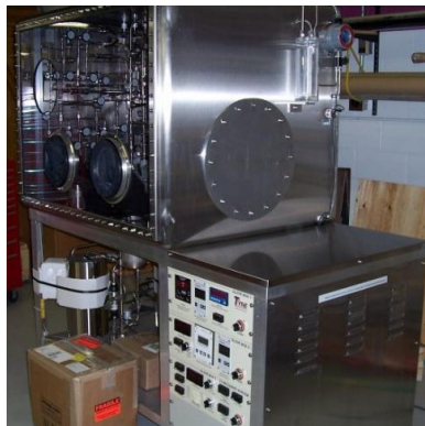
Leak Proof Glove Box and Controls Electronics Designed and Manufactured by Tyne Engineering
