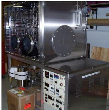
Leak Proof Glove Box and Controls Electronics
